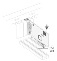
Figure 2-3: Aligning the card against the slot.
